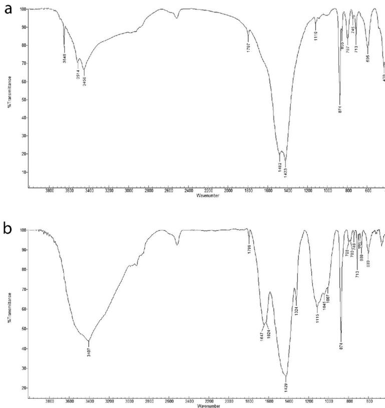
Figure 2 FTIR transmittance spectra of the stucco layer of sample 4 (a), showing the co-presence of calcite ( $874, 713 \text{ cm}^{-1}$ ), magnesite ( $744 \text{ cm}^{-1}$ ) and hydromagnesite ( $3649, 3512, 3447, 1428$  and  $1423 \text{ cm}^{-1}$ ), and of the finishing layer of sample 1 (b), showing the presence of weddellite ( $1647$  and  $1324 \text{ cm}^{-1}$ ).
