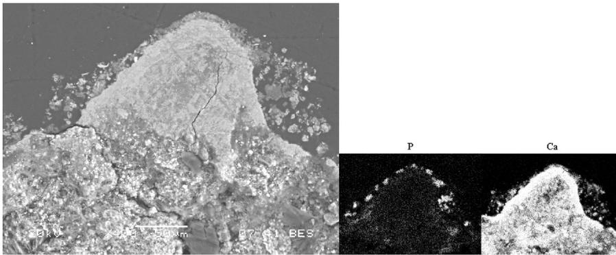
Figure 7 Polished cross section of sample 4 analysed by SEM-EDS. Backscattered image of polished cross section (left, bar 50µm), EDX distribution maps of P and Ca of the same area (right).
