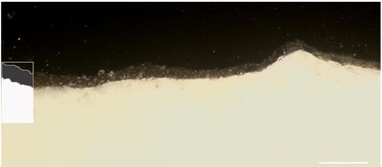
Figure 4. Polished cross section and stratigraphic scheme of sample 1 (bar 100 µm) showing the presence of just one finishing layer.
